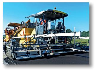
components of an asphalt finisher include a tractor or other such machine to drive it forward, an engine including hydraulic drives and controls, either drive wheels or, a hopper for receiving the asphalt, feeder conveyors and distribution augers.
