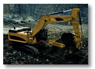
hydraulic systems. Beneath the rotation point (slewing ring), excavators may be mounted on either a crawler (tracked) or wheeled undercarriage.
