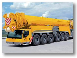
mounted cranes, but are differentiated by large tyres to provide ground clearance and off-road mobility, a multi-axle chassis and all-wheel drive and steering.
