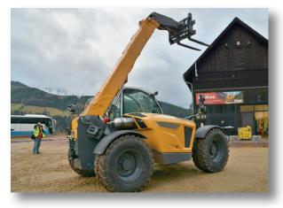
industrial forklift truck – or a telescopic boom. The latter are often called telescopic handlers or simply telehandlers. Telehandlers can be fitted with a variety of attachments, including pallet forks, bucks and access platforms, which combine with their vertical and horizontal reach capabilities to provide a versatile machine
